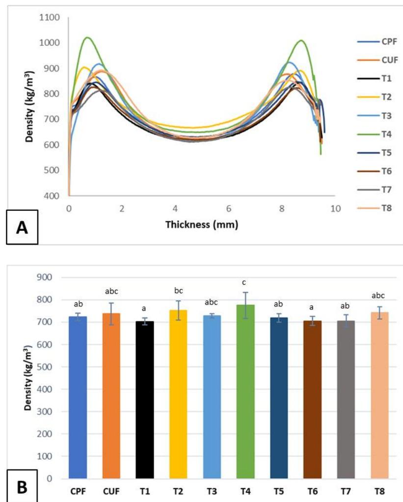
**Figure 4.** Density of the MDF residue-PCM panels. (A) The VDPs of the manufactured panels; (B) the average density of the manufactured panels according to the QDP-01X densitometer. The panel type acronyms are defined in Table 2. The lowercase letters represent statistically significant differences between panel types according to the Tukey test.
