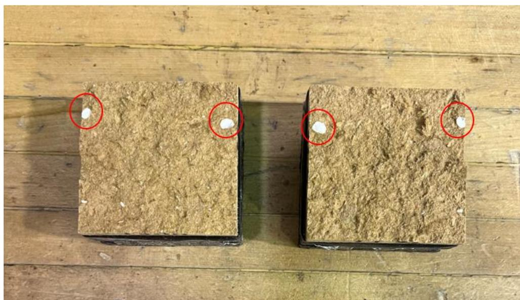
**Figure 7.** MPCM aggregates formed during panel fabrication.
