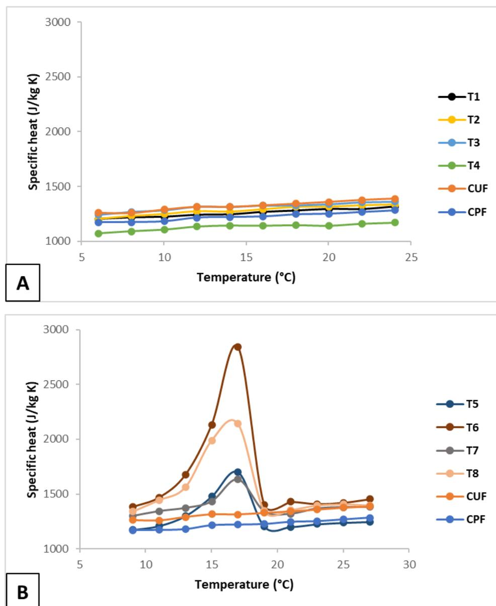
Figure 9. Specific heat of the panels. (A) Panels made with PCM1; (B) panels made with MPCM.
