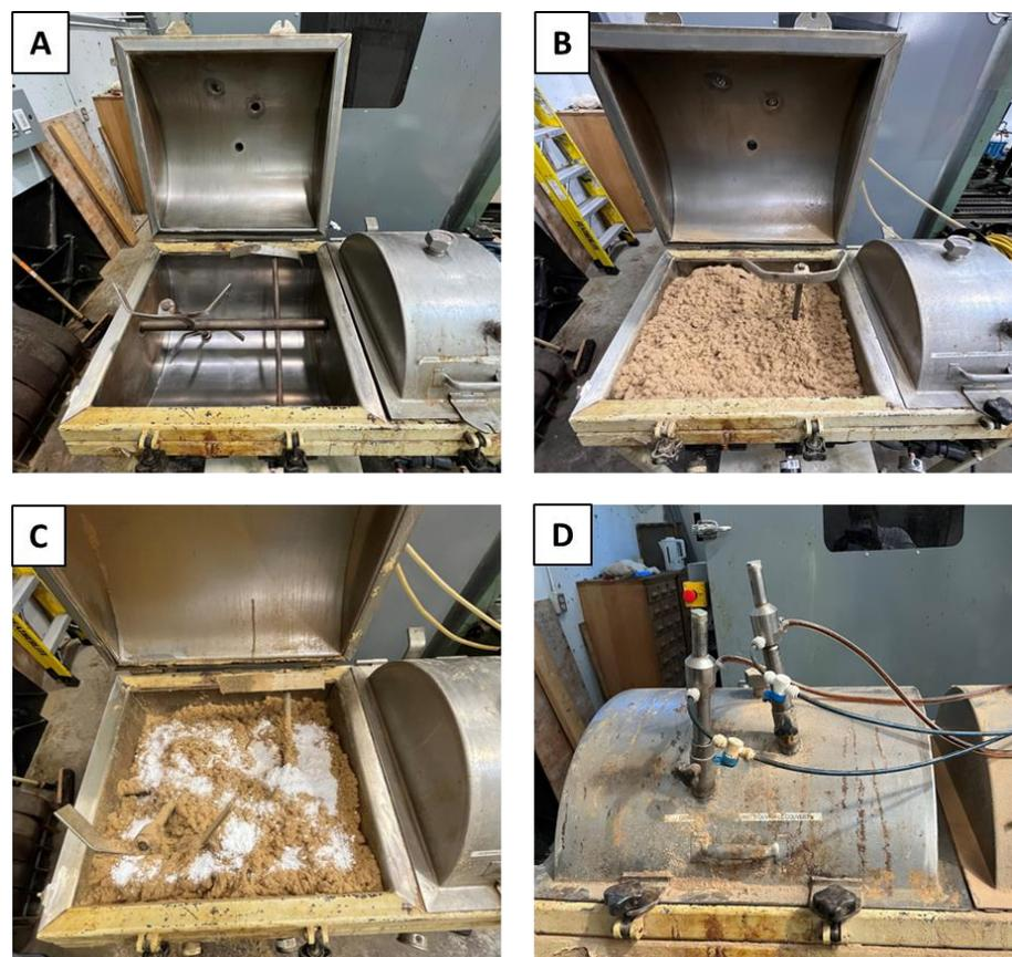
**Figure 1.** House-made horizontal blender. (A) The rotating blender blades; (B) the MDF residues before blending; (C) addition of MPCM to the MDF residues before blending; (D) the system used for spraying and incorporating the adhesives and PCM1.
