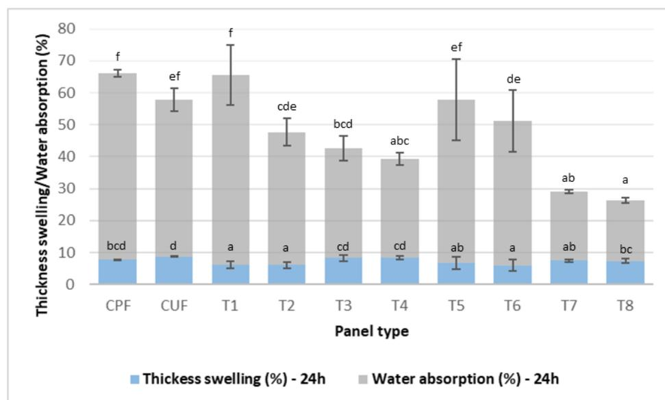
**Figure 5.** Thickness swelling and water absorption after 24 h immersion in water. The panel type acronyms are defined in Table 2. The lowercase letters represent statistically significant differences between panel types according to the Tukey test.
