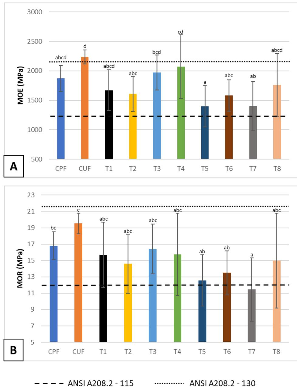
**Figure 8.** Static bending properties of the panels. (A) MOE; (B) MOR. The lines represent the requirements that are set out in ANSI standard A208.2 for MDF. The panel type acronyms are defined in Table 2. The lowercase letters represent statistically significant differences between panel types according to the Tukey test.
